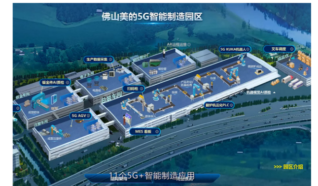
▲ Panoramic view of Midea's 5G smart factory. 20,000+ data collection points were deployed in the campus, integrating various technologies to create a 5G+UPF+MEC solution to enable 11 5G+ industrial Internet application scenarios
